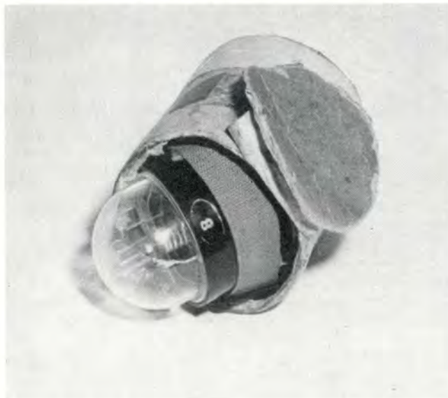
Hydrogen generators, the gadgets that blow up the antenna balloons are unusable. The small signal lights are being crushed and cracked.
