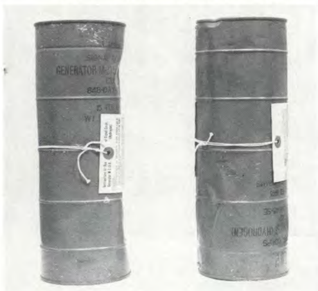
Hydrogen generators, the gadgets that blow up the antenna balloons are unusable. The small signal lights are being crushed and cracked.
